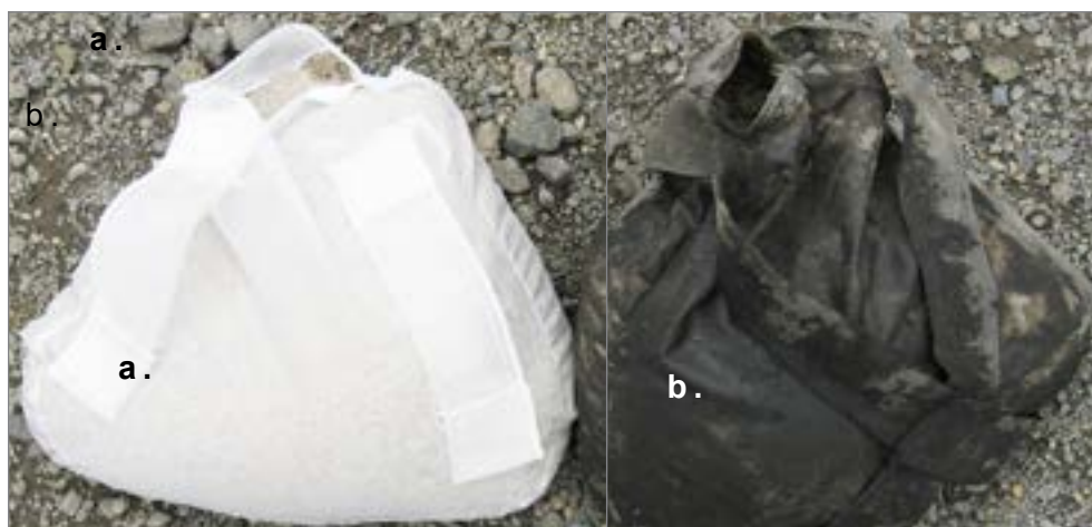
Fig.4 a) A new Media Bag of Hydro Filter Sand. b) A spent media bag of Hydro Filter Sand.
